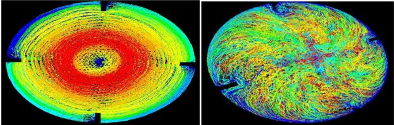
**Figure 7: Pathlines at the top and bottom face of the slurry tank**
