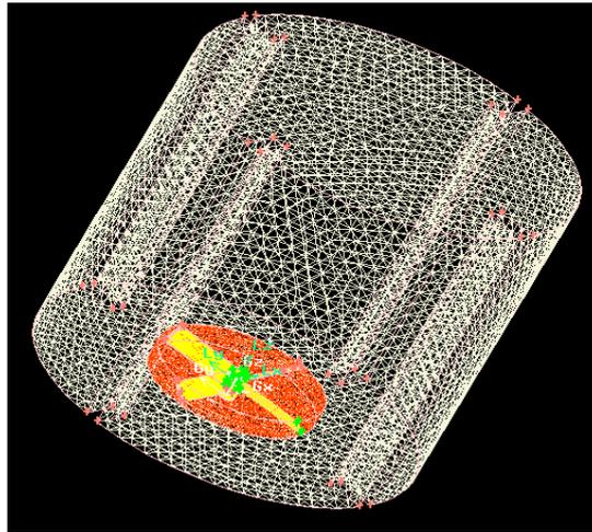
Figure 5 : Mesh of Tank, Impeller and Rotating Frame
