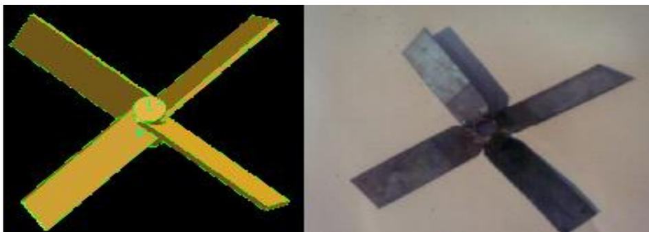
**Figure 2 : a) CAD model of the Impeller, b) Impeller**
