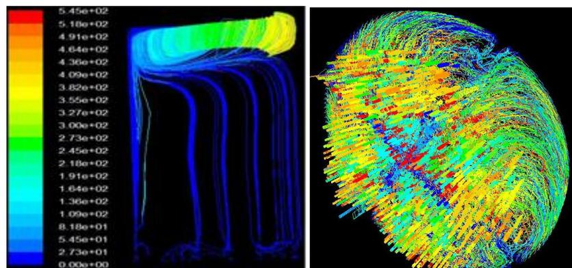
Figure 6 :Pathlines of fluid at bottom face inside slurry pot, shown in the left portion of the Y-Z plane
