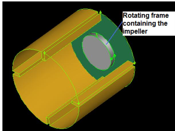
Figure 4: Slurry pot model with rotating frame
