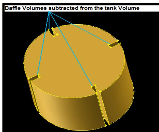
Figure 1: Fluid Volume excluding baffle space
