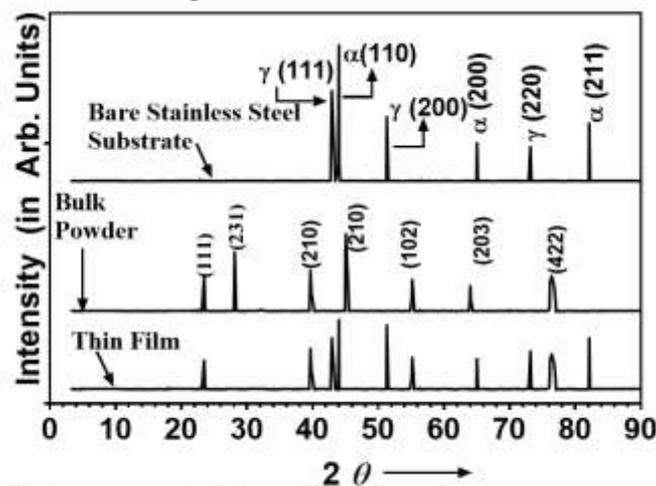
Fig. 1. A typical XRD of Bulk powder and as-grown CdSe<sub>0.4</sub>Te<sub>0.6</sub> thin film on stainless steel substrate
