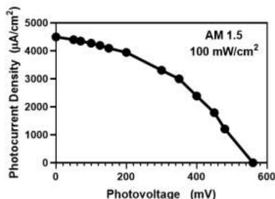
Fig. 3. Power Output Characteristic of  $CdSe_{0.4}Te_{0.6}/(aq)$  Polysulphide PEC Solar Cell.
