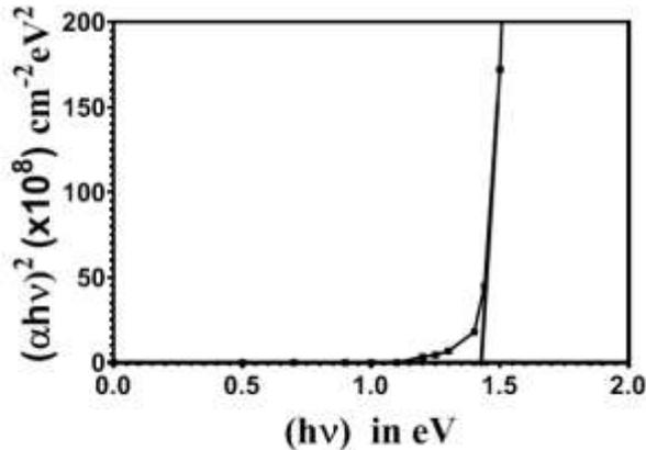
Fig. 2. A plot of  $(\alpha hv)^2$  vs  $(hv)$  for an as grown  $CdSe_{0.4}Te_{0.6}$  thin film on stainless steel substrate.
