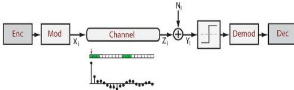
Figure 1: Simplified model of a high-speed link. Transmit / receive equalization is reflected on the symbol-spaced pulse response.
