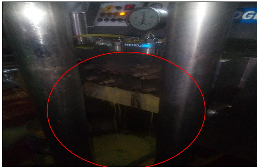
Figure 2.1: Leakage occurred from Compression head because of Hair line crack on its surface with SS 316L grade of material
